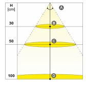
VERS. NW A° 80° B - Lux 670 C - Lux 270 D - Lux 80 LUMEN 180 LUMEN / W 60 CRI >80
